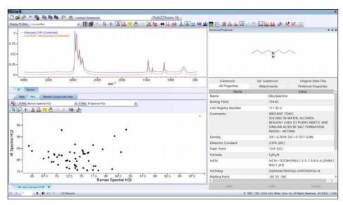
For example: This plotting feature is useful in the analysis of spectral searches for samples run in multiple techniques by plotting the quality of database search results (Hit Quality Indicies - HQIs) against each other (e.g., IR HQI versus Raman HQI).
