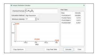
**Isotopic Distribution Calculator.** Calculate the isotopic distribution from a chemical formula using either low resolution or high resolution to a user defined threshold.
