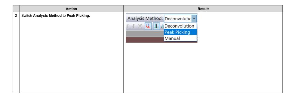
Action Result Reduce the **Sensitivity** to **Low** so that only main peaks are MS Expert • 🖩 🗗 🛚 picked (A). Select the peak at 3.8917 min. RT [min] # # Match 2.3778 # 1 Barbital 3.8917 # 1 Butethal Score HQI R.H., Notes 93.27 93.24 93.48 92.69 92.39 95.45 Hold the mouse cursor over the solid square denoting the 4.2577 ⊞ 1 2,4,6(1H,3H,5H)-Pyri 4.4133 ⊞ 1 Amobarbital 4.6077
